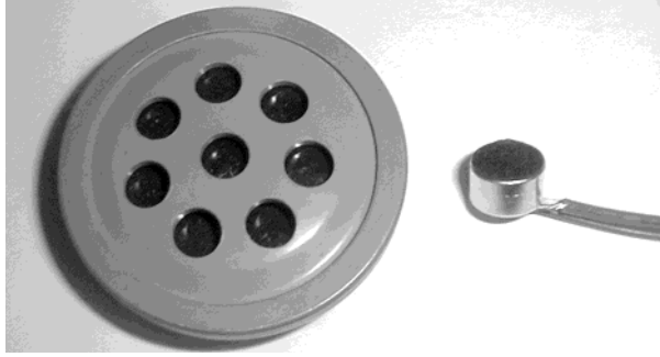
Fig. 1-4. Carbon (left) and electret (right) microphones
