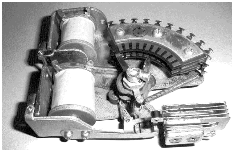
Fig. 11-4. A small stepper relay
